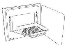
The Handyrack fits to the left hand Main Oven door only. Food cooking on it is easy to attend to, because it's accessible when the door is open. It can be fitted at two different heights. One of the oven shelves must be removed and the other positioned to suit.
